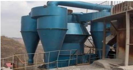
The sugar Industry produces power for in-house consumption and the surplus power is sold to national grid. Improving the use of fuel i.e. Bagasse in the boiler is an important industrial approach for more earnings of the sugar industry. By use of Bagasse driers, boiler efficiency can be increased considerably on account of reduction of Bagasse moisture.
