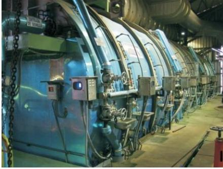
Continuous vacuum pans have now established their position in the sugar Industry. They provide significant advantages such as minimal supervision, benefits to steam economy, better exhaustion, crystal uniformity, etc. The most important criteria for a successful Continuous Vacuum Pans are production of even crystal size, elimination or avoidance of encrustation, lump formation and energy usage. Major advantages are:
